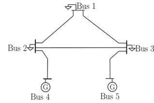
Fig. 2. A 5-bus system ([17], Chapter 6, pp.327). In this system, we assume that each bus has a battery attached to it.
