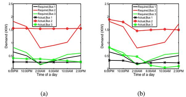
Fig. 3. Actual and required demand under different  $\alpha_i \forall i = 1, 2, 3$ . (a)  $\alpha_i = 0.01$  (b)  $\alpha_i = 0.1$ .
