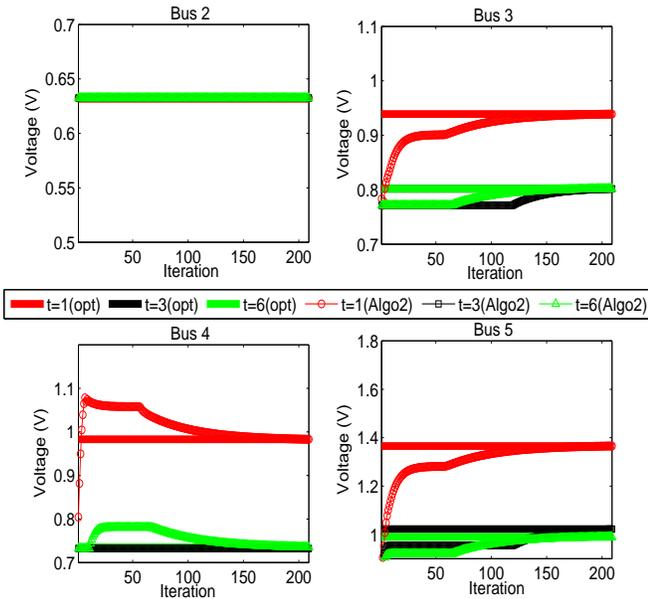
Fig. 5. Illustration of convergence of Algorithm 2 in the 5-bus system with the initial point set further away from the optimal solution.
