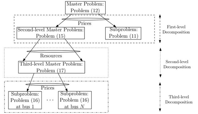
Fig. 1. Indirect optimization decomposition to solve the OPF with energy storage problem in (7). The partial dual decomposition, the primal decomposition and the partial dual decomposition are applied in the respective three levels.
