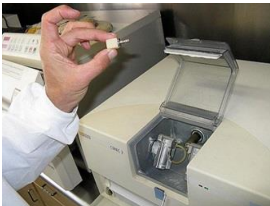
FIGURE 3 :The CEREC 3 system (Sirona) can fabricate inlays, onlays, crowns and the cores/frameworks of fixed dental prostheses.
