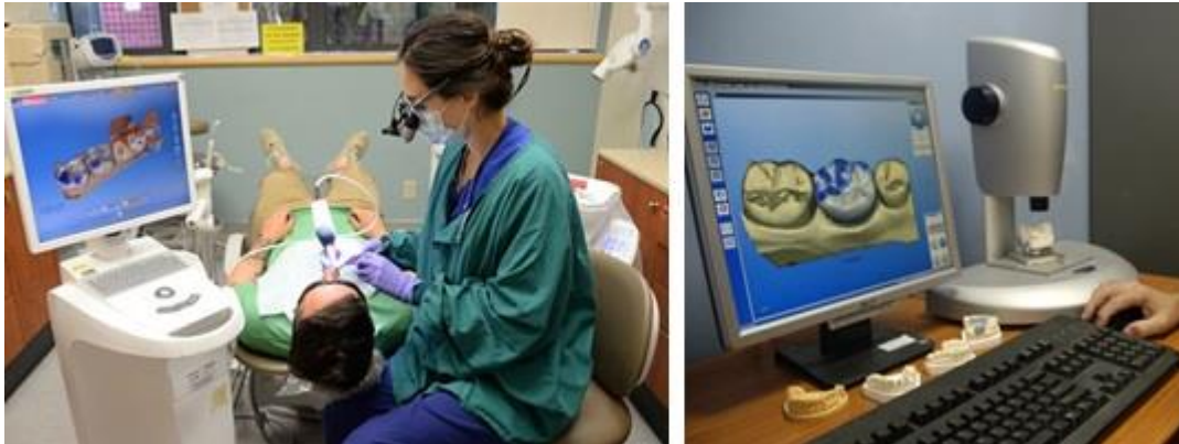
FIGURE 2: A digital impression system consisting of an intraoral scanner connected to a workstation with a computer display; A virtual model is obtained through the scan on which a prosthesis can be designed.
