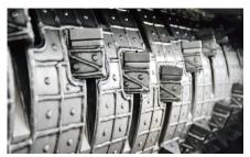
The ZTS and ZTTS shredders are equipped with large diameter flat rotors with weld on hard facing. The knives are fixed in special knife holders fitted in machined pockets.
