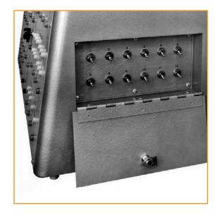
The fault-creating feature of these controllers is particularly useful in developing troubleshooting techniques as well as reinforcing the regular study of motor control theory. Twelve program switches are located behind a locked panel on the side of the controller. With these, the instructor may inject any combination of up to 12 faults into the controllers wiring. The faults are designed to be typical of ones normally encountered in electromechanical systems.
