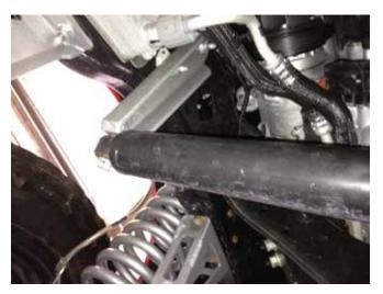
26. Install steering shock stud into the original track bar and tighten to factory specifications.
