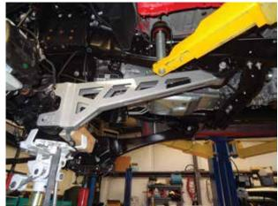
2. Use the provided bolt with alignment cams for the front lower hole with "D" shape washer and lock-nut.
