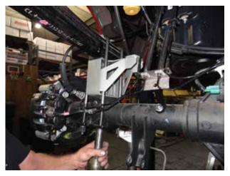
36. Install new rear shocks into the factory location. The body of the shock goes towards the ground (bottom mount which is on the rear-end housing) and the top shaft of the shock goes to the frame.
