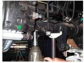
33. Use a C clamp and clamp the leaf clamp together at each end so that when you remove the leaf spring center bolt the spring does not come apart.
