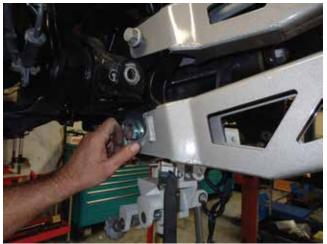
4. The four, 4-link arms are all specific to the side they fit on and their location. The two lower arms have the name plates. You can determine the driver and passenger side by the McGaughy name plate. The McGaughy nameplate should be facing outwards. The upper 4-link arms have a small hole drilled about in the middle (front to back middle). The hole is for the ABS sensor wire but don't install the sensor yet.
