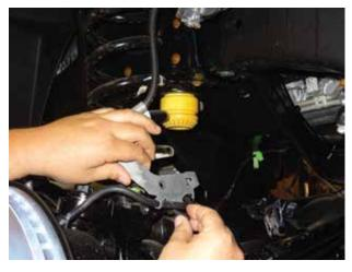
3. Remove the bolt in the frame that holds on the steel brake line bracket for the steel brake lines so that the brake lines are not bolted to the frame. (both sides)
