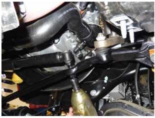
9. Loosen the upper factory mount of the track bar (on the driver side) and let it hang down.
