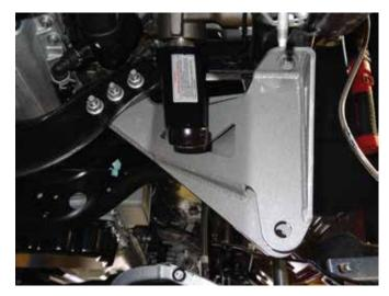
20. Install the new driver and passenger side bump stop brackets. The brackets are the same and don't matter which side they go on. The bump stop bracket bolts under the frame to the hole that you already opened up from step #16. Use the provided 3/8" x 1 1/4" bolt to install the bracket to the frame. Bolt the black retainer to the new drop bump stop bracket using the provided 5/16" x 1 bolt.
