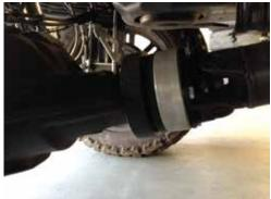
38. Check all hardware and make sure everything is tight. Check for clearance on all parts to make sure that there won't be any rubbing on brake lines, sensors, clips, tires, etc. Make sure you go to a reputable frontend shop to get an alignment. After 500 miles re-check and tighten all parts.
