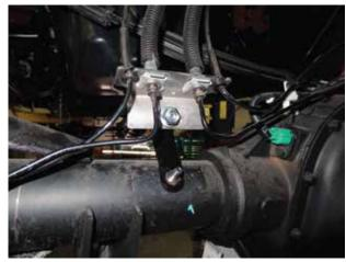
32. Make sure the rear-end is supported so that it can't move or twist. Remove the factory U-bolts and factory lift block.
