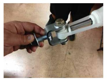
23. Install the stock, front track bar to the track bar drop bracket. You use the factory hardware and the bottom hole of the bracket.
