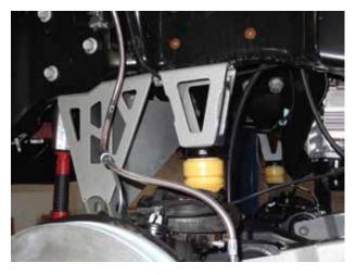
21. Install the new McGaughy's lift coil. The pig-tail on the coil goes to the bottom (closest to the ground). There is a specific driver and passenger side coil on the 8" lift kit. The 6" kit does not matter which side the coil goes onto and is not side specific.
