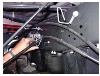
31. Remove the rear-end vent tube from the vent fitting on the rear-end. Remove the factory brake line bracket from the rear-end housing. Un-bolt the vent tube bolt (the one that holds the brake line bracket to the rear-end housing). Use provided brake line extender bracket and the original vent tube bolt to bolt the bracket to the rear-end housing. Bolt the brake line bracket to the other end of the new brake
