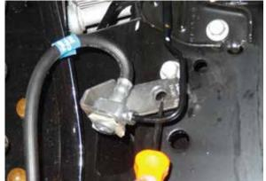
4. Disconnect the sway bar end links (The truck has one on the driver side and one on the passenger side).
