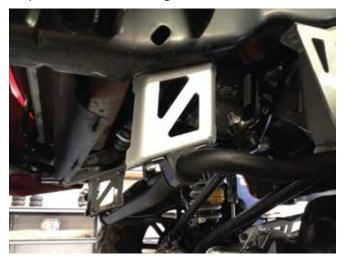
28. Install the sway bar onto the new sway bar drops with the new  $3/8'' \ge 1/2''$  bolts and hardware. Reinstall the sway bar end links into the front axle but don't connect to the sway bar until the truck is stiing on the ground.
