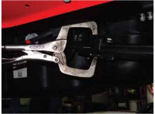
34. Remove the emergency brake clip from the leaf spring center bolt.
