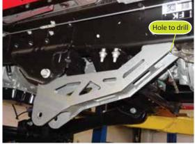
2. Use the provided 18mm bolt to bolt the factory radius arm to the front of the new mount from the previous step.
