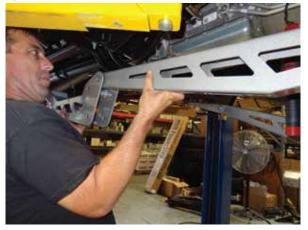
2. Bolt the 4-link lower arm to the new drop bracket (the bottom front hole on the drop bracket) using the provided  $3/4'' \times 5''$  bolt.
