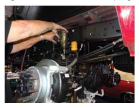
**ONLY If you have an 8" Kit:** Install the new add-a-leaf between the over load leaf and the bottom leaf. Use new provided center bolt. Make sure you use clamps to suck the leaf pack together, don't rely on the center bolt to close the gap. Before you tighten all the way down, install the new provided U-bolt retainer plate. You will not use your original U-bolt retainer plate. Make sure leaf spring center pin is tight.
