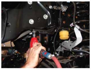
12. Use a 46mm socket to remove the pitman arm nut.
