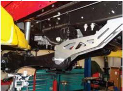
16. Using a uni-bit, open up the front factory bump stop hole so that a 3/8" bolt will fit.
