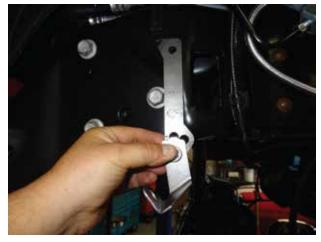
18. Install the new McGaughy's pitman arm using the factory nut and tighten to factory specifications. Use Lock-Tite on the factory nut.
