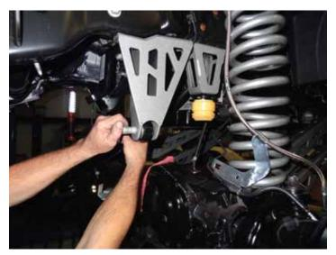
24. Install the stock drag link into the new drop pitman armand use the original hardware including the castle nut and cotter pin. Tighten to factory specifications.
