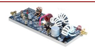
The RFP13.56-100XR is a high gain Class A/AB XR-rated amplifier designed specifically for the 13.56MHz ISM band. It is ideal as a driver stage or output PA in high power industrial, commercial, or scientific systems. Its XR rating ensures ruggedness when driving mismatched loads such as plasmas. It is supplied with SMA input and output connectors.
