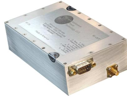
The RFM20-512-100-HSD is a Class A/AB high performance amplifier module, excellent as a driver stage in military communication or radar systems. It features fast output disable with  $\leq 1\mu\text{sec}$  response time. An independent MMIC disable line affords additional quieting of the RF chain. It utilizes a combination of three active device technologies for optimum performance and maximum ruggedness.
