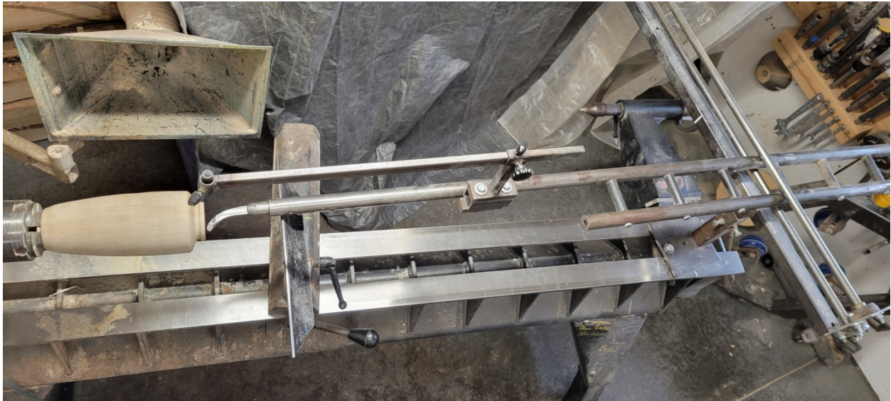
This is my own personal 1 1/4" trapped boring bar; I use the curved cutter with the adapter so I can easily change from tool to tool.
