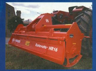
New trailing board with curved profile to break up soil better and prevent it from sticking under moist conditions. Models from 130 cm. up to 205 cm. with standard top mast and double tube.
