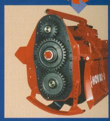
Detail of the side drive gears, in models HR16 and HR21.
