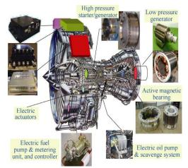
Fig.3. Power optimized aircraft engine
