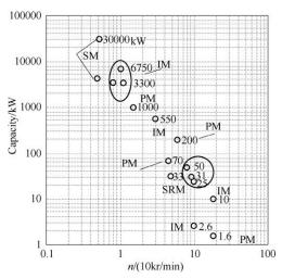
Fig.5 Nominal output power versus rotation speed of some of the prototyped and or manufactured high speed machines
