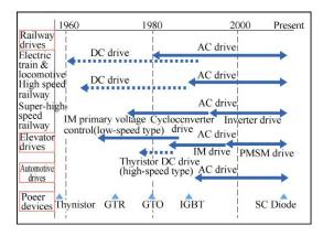
Fig.1 An overview of transportation motor drive technologies and products in Japan
