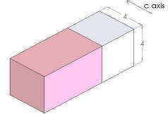
**COATING** Both ends R<0.05% @ 1064nm, R<3.0% @ 808nm
