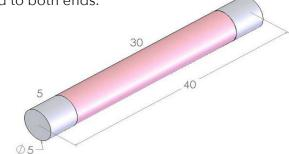
**COATING** Undoped YAG: R>99.9% @ 1064nm, Tav>97% @ 790-820nm, AOI = 0-50° Nd:YAG: R<0.15% @ 1064nm, Tav<3.0% @ 790-820nm, AOI = 0-15°
