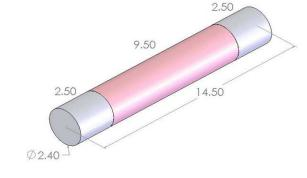
**COATING** Both ends R<0.1% @ 1990nm, AOI = 0°, R<1.0% @ 795nm, AOI = 0.0+/-12.5°
