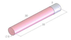
**COATING** Undoped YAG: R>99.9% @ 1064nm, Tav>97% @ 790-820nm, AOI = 0-50° Nd:YAG: R<0.15% @ 1064nm, Tav<3.0% @ 790-820nm, AOI = 0-15°
