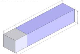
**COATING** Both 3.0 mm x 3.0 mm end faces R<0.15% @ 1064nm and R<3.0% @ 880nm
