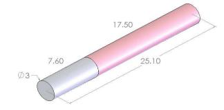
**COATING** Nd:YAG end: R<0.25% @ 1064nm, Undoped YAG end: R<0.25% @ 1064nm, T>98% @ 808nm
