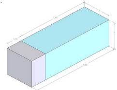
**COATING** Both 3.0 mm x 3.0 mm end faces R<0.1% @ 1064nm and R<1.0% @ 808nm
