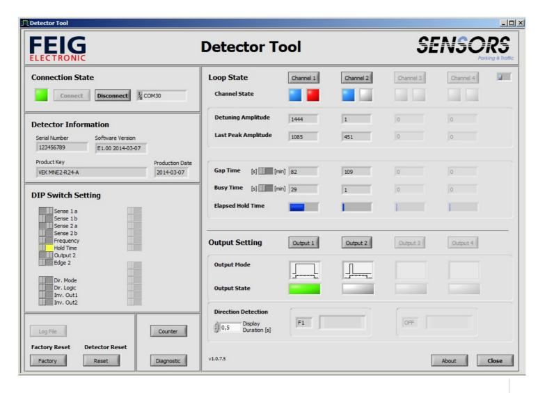
The USB interface of the detector allows connection to a PC, notebook or Tablet PC. With the help of a diagnostic and service software, the existing configuration of the device can be shown and conveniently changed directly on site.
