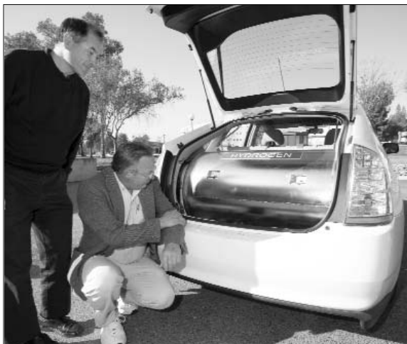
Salvador Aceves (left) and Tim Ross check out the on-board hydrogen storage tank. Photo by Jacqueline McBride/LLNL
