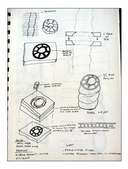
This model explores tube compression by using a double-membrane made of silicone. The goal is to look at how the muscle membrane reacts. Exercises include varying the spacing of the stacked units and variation of the shape — circular, square and rectangular. Could this be combined with fluid & heat activated wire? Perhaps hot water heats the water and provides movement. To illustrate model working video could zoom
