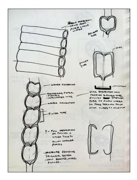
The "Foam" one deals with milling out C-shapes that combine in a mold and are connected with a wire so that when the wire is pulled it causes a reaction in the material, causing the C-shapes to separate. Could possibly use a rubber gasket to create a seal to keep the water from seeping through when the wire is not pulled taut. Shapes will be made out of liquid foam. It is porous and retains the shape created.
