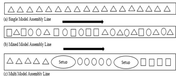
Figure 4: Assembly lines for single and multiple products **iii). Multi-Model:** In this model the uniformity of the assembled products and the production system is not that much sufficient to accept the enabling of the product and the production levels [7]. To reduce the time and money this assembly is arranged in batches, and this allows the short term lot-sizing issues which made in groups of the
