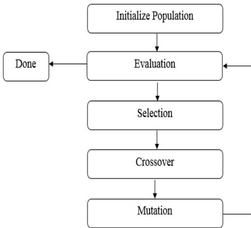
Figure 6: Flow chart of genetic algorithm
