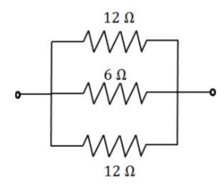
2) Find the current through each resistor, the potential difference across each resistor, the power being delivered by the battery and the power dissipated by each resistor.
