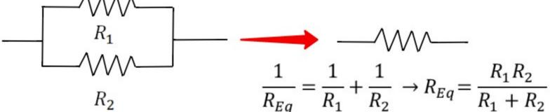
$$R_{Eq} = \frac{R_1 R_2}{R_1 + R_2}$$
