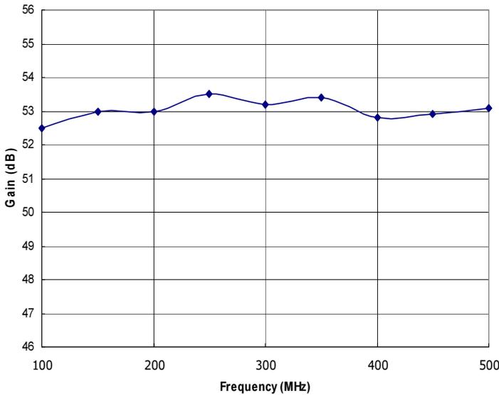
Figure 1: RFM100-500-100-HSD Typical Gain @ P<sub>out</sub>=100W.
