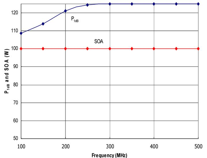
Figure 4: RFM100-500-100-HSD Typical P<sub>1dB</sub> and Safe Operating Area (SOA). Do not exceed the SOA shown above without first contacting RFMPT to discuss your application.
