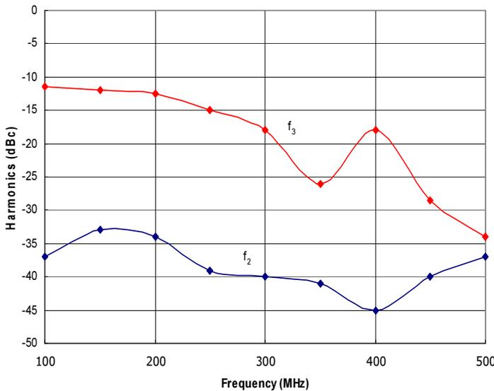
Figure 3: RFM100-500-100-HSD Typical f<sub>2</sub> and f<sub>3</sub> @ P<sub>out</sub>=100W.
