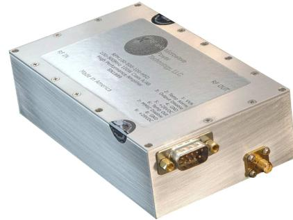
The RFM100-500-100-HSD is a Class A/AB high performance amplifier module, excellent as a driver stage in military communication or radar systems. It features fast output disable with  $\leq 1\mu\text{sec}$  response time. An independent MMIC disable line affords additional quieting of the RF chain. It utilizes a combination of three active device technologies for optimum performance and maximum ruggedness.
