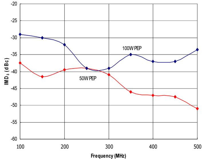
Figure 2: RFM100-500-100-HSD Typical IMD<sub>3</sub> @ 100W and 50W PEP, Δf=10kHz. For improved linearity, see our RFM100-500-50-HSD Class A amplifier.
