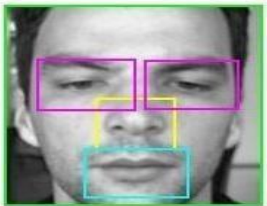
Figure 10: Face features (parts) identified by Voila-Jones algorithm (Boundary box).
