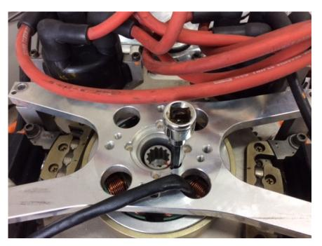
The final result should Allow flywheel bolt torque with an extended 1/4 inch hex driver (same one used on bottom head bolt).
