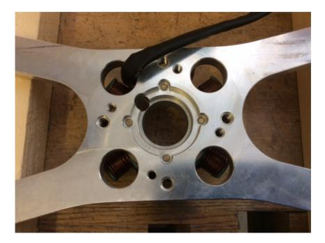
Next: Carefully drill through the stator mount and stator spacer
