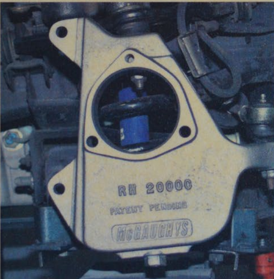
6. McGaughy's new drop spindle, PN 2000C, was installed and tightened.
