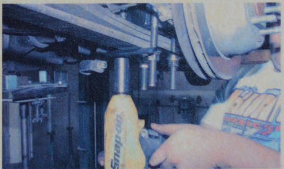
13. To wrap up the rear, Mike tightened the U-bolt nuts and reinstalled the wheels and tires.
