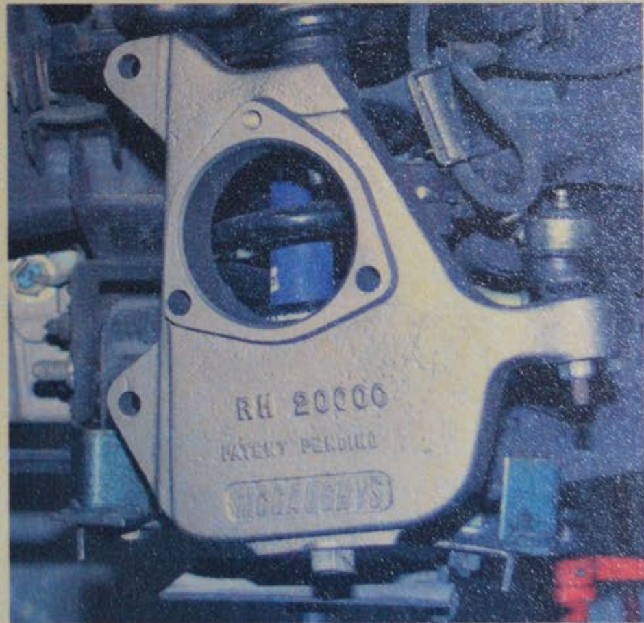
7. With the tie rods and the upper and lower ball joints attached, it was time to move to the hub bearing.
