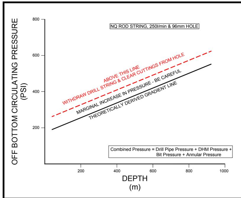
**Figure 8.** Monitoring off-bottom pressure can be used as a guide to drilling practice.
