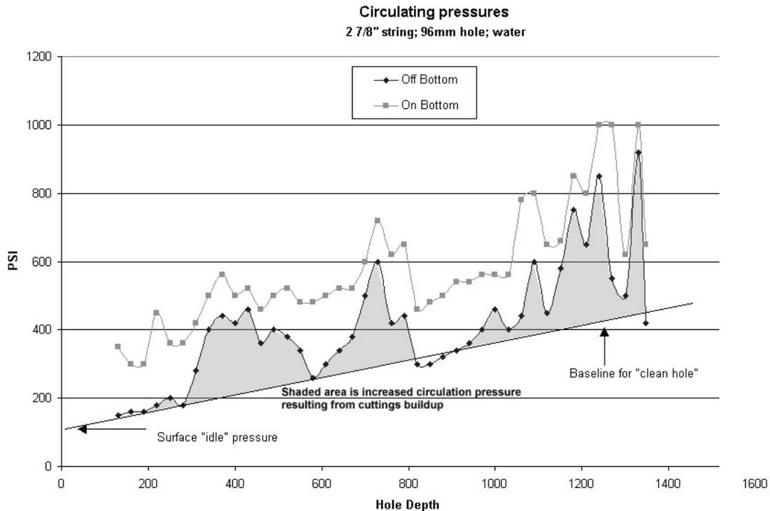
**Figure 7.** Monitoring off-bottom pressure can improve the understanding of circulation issues and geological problem zones (from Thomson & MacDonald, 2002).
