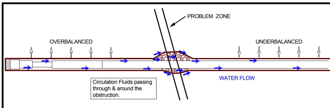
**Figure 4.** Differential sticking is a leading cause of stuck drill pipe in underground in-seam drilling.
