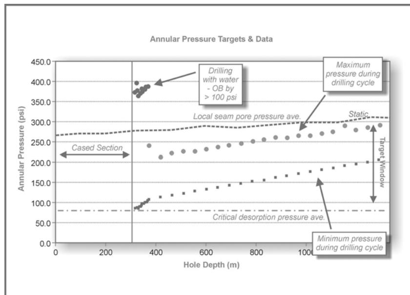
**Figure 4.** The importance of maintaining balance in drilling is exemplified by this surface to seam example from Queensland (from Thomson & MacDonald, 2003).
