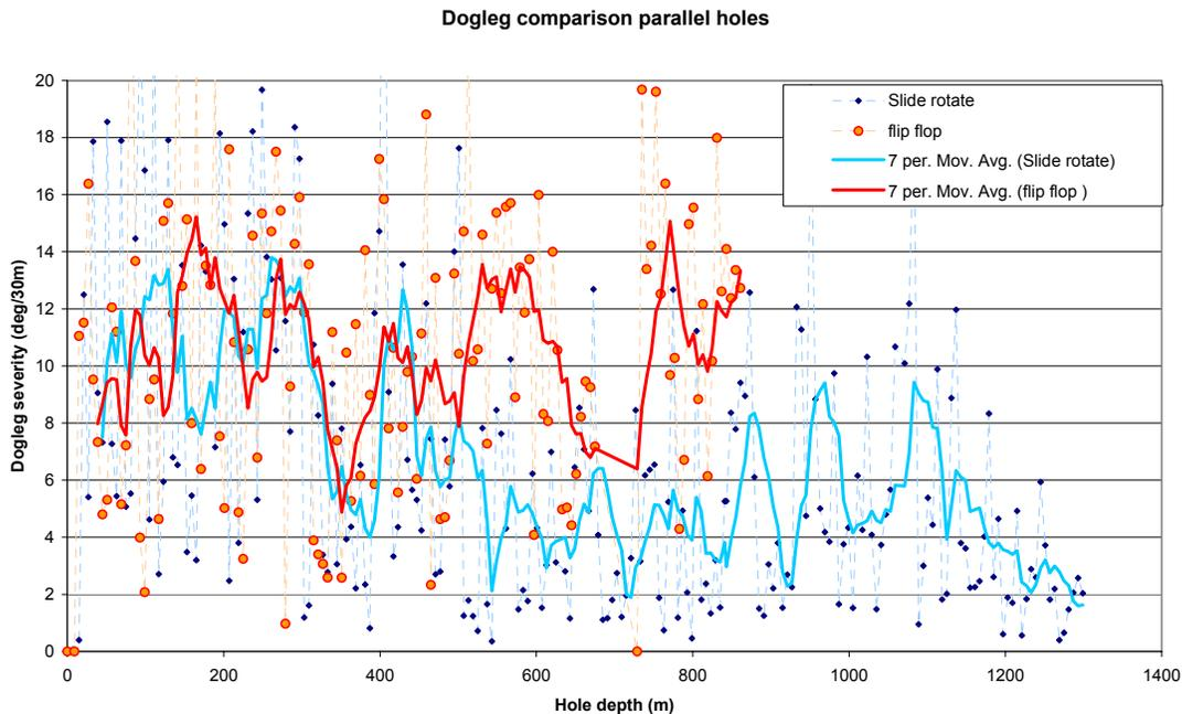
**Figure 3.** Dogleg severity in two parallel boreholes, one drilled entirely with the 'flip flop' method (Hole 1) and the other with mainly 'slide / rotate' (Hole 2).
