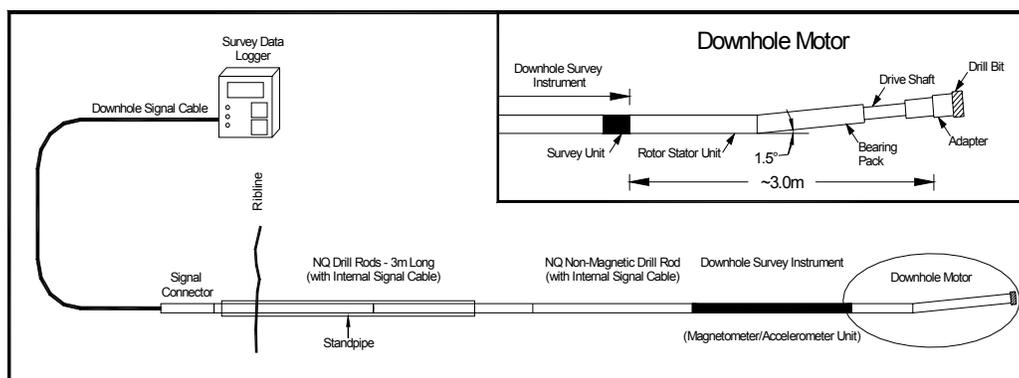
**Figure 1.** Schematic representation of standard practice directional drilling downhole equipment
