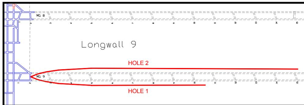
**Figure 2.** Comparison of two parallel boreholes, one drilled entirely with the ‘flip flop’ method (Hole 1) and the other with mainly ‘slide / rotate’ (Hole 2), (Thomson, 2001).
