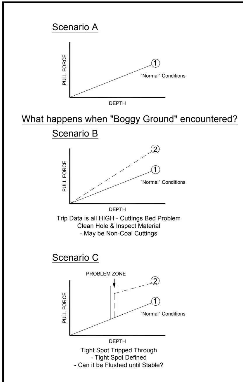
**Figure 6.** During string withdrawal pull force may be monitored to determine the position of problem zones in the formation
