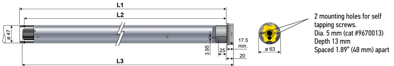
2 mounting holes for self tapping screws.
