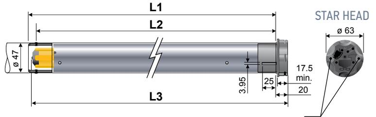
2 mounting holes for self tapping screws. Dia. 5 mm (cat #9670013).
