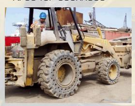
Applications: Rental Fleets, Construction, Outside Demolition. All purpose soft-ride solid tires for use on and off road. Full size construction, deep lugs, excellent traction in dirt, extended life on hard surfaces and reusable rims.
