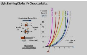
Light Emitting Diode (LED) Schematic symbol and I-V Characteristics Curves showing the different colours available.
