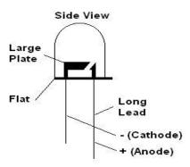
Scientifically to emit light from led the process by which lasers work is reversed. we make the electron fall from higher to lower energy level. This phenomenon is exploited in led. Red or yellow light is produced by using Gallium-Arsenide-Phosphorus (GaAsP) as a semiconductor. Red or green light is produced by using Gallium-Phosphorus (GaP) as a ISSN: 2454-7301 (PRINT) | ISSN: 2454-4930 (ONLINE)
