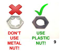
9. It is now time to fasten the LED ring and button to the cabinet using the included PLASTIC Pal nuts. IMPORTANT: <u>DO NOT USE THE</u> <u>OLD METAL NUT TO SECURE YOUR LED BUTTON LIGHT</u>. The metal Pal nuts can conduct electricity and short circuit the LEDs! Only use the included plastic Pal nuts to secure your LED ring and new button.
