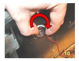
10. Apply the included plastic pal nuts to the button shafts, turning clockwise. They should be hand tight, but <u>do not use excessive force</u> <u>as this can damage the LEDs</u>. A very small amount of tightening with pliers can be used beyond hand tightening. But do not go much beyond hand tightening. The plastic nut fitment and notches in the cabinet will prevent the buttons from being loose or spinning.
