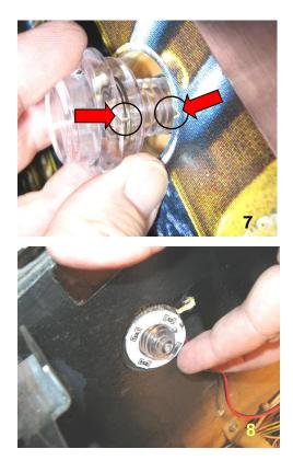
7. Fit the new, clear buttons into the cabinet flipper button holes, making sure to align the notches on the rim of the button with the notches on the cabinet hole. Some cabinets have notches that are very pronounced, others do not. The button may require a few taps in with a soft mallet if the fit is snug.
