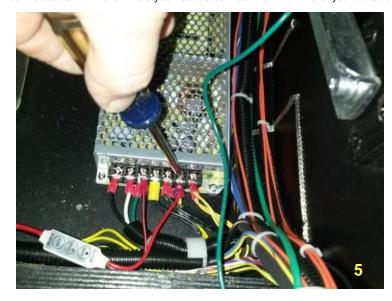
5. Once the red and black wires from the BriteButton kit are connected to the Ground and +12V power supply terminals of your pinball machine (as illustrated) you can replace the clear plastic protective cover and two screws.
