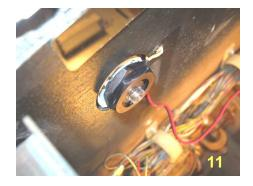
11. For some machines, only one Pal nut is possible to fit on the button threads. This is due to the different countersinking depths of various wood cabinets. If two Pal nuts can fit on the button, a second set is provided and may be used to help prevent excess light leakage from the button into the cabinet. Do not over tighten.
