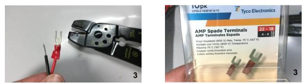
3. To connect your red and black wires from the BriteButtons to the power terminals of your MMR pinball machine, you can "tin" the stripped wire leads with a little solder, or add 22-18 spade type crimp thermals (recommended), available from your local hardware store.
