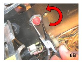
6A. Perform the following for both pairs of flipper buttons. In some cases your flipper buttons can be replaced without removing the flipper switches (opto assemblies). However, it is best practice to first remove them if possible so you can fully access the buttons without damaging the switch parts. 6B. Remove the old Pal Nut by turning counter-clockwise. If tight, small needle nose pliers can be expanded within the Pal nut rim and used to turn the nut. Remove the old flipper buttons.
