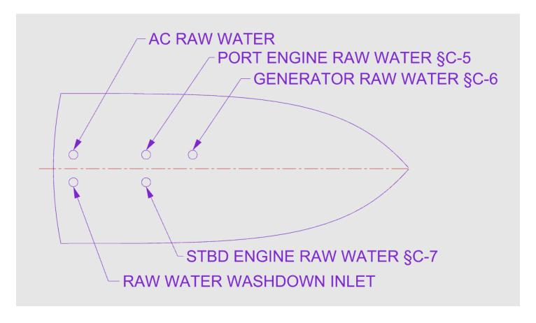
§C-5, 6 &7 Ball valves are stuck in the open position.
