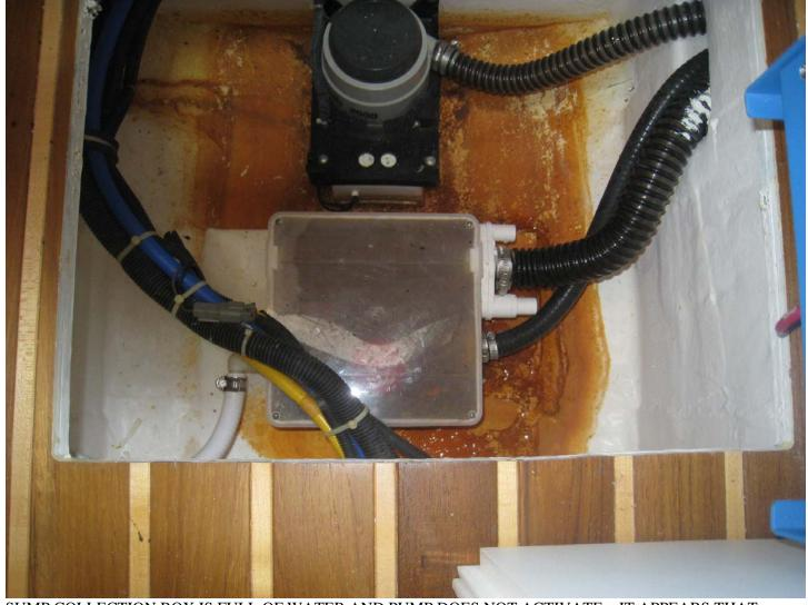
SUMP COLLECTION BOX IS FULL OF WATER AND PUMP DOES NOT ACTIVATE. IT APPEARS THAT WATER COLLECTS IN THIS AREA. THE RUST APPEARS TO COME FROM THE AIR CONDITIONING CONDENSATE. WHEN ENOUGH WATER COLLECTS, IT IS EMPTIED BY THE BILGE PUMP.
