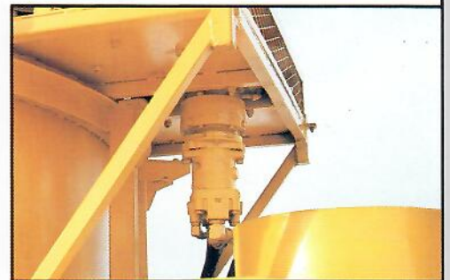
The tub is driven by a Sundstrand planetary gear with a ratio of 22:1.
