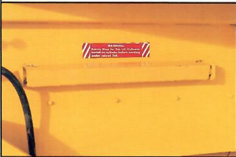
A conveniently-mounted safety brace is used to lock tub in the "up" position during servicing.
