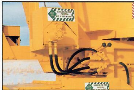
Hydraulic controls for elevating, lowering or folding the conveyor are located within easy reach.
