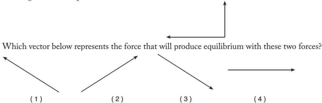
9. In the diagram below, a 20-newton force due north and a 20-newton force due east act concurrently on an object, as shown in the diagram below.
