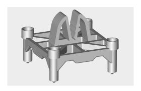
**Art Mould's Precast Chair** is a versatile **Stackable Chair** with a single clip that fits mesh to 20M bar. It is made with composite material for strength, corrosion resistance and durability, while the design allows for concrete flow, and eliminating the risk of voids. Its pointy legs result in minimal contact and exposure on the panel surface.
