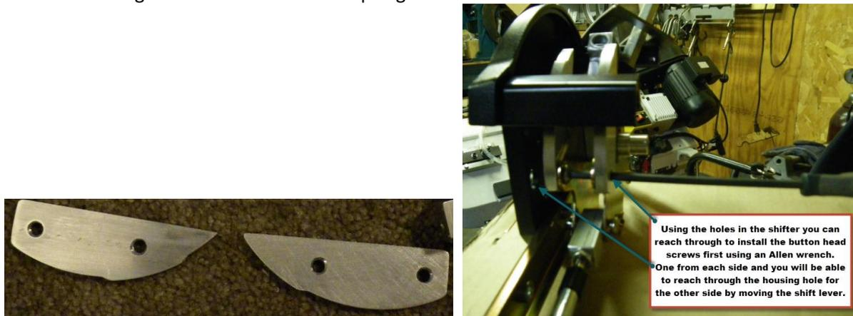
Next install the shift switch brackets one on each side using the existing threaded hole in the shifter frame, check to be sure they are switching on and off as you move the shift lever.:
