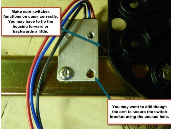
Now reassemble your shifter and connect the wires as marked, make sure your 12V+ supply is on a key on fused source. The two connected black wires are for your 12V+ supply.
