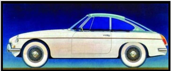
The MGB GT's windshield is about 4 inches (101 mm) taller than that of the roadster while the side windows are about 1.5 inches (38 mm) higher; the front fenders were reshaped to maintain the car's proportions. The GT had the same engine as the roadster, a 1,798 cc (110 cu. in.) B-series four making 98 hp (73 kW) and 110 lb-ft (149 N-m), but the coupe's extra weight makes it a bit more than a second slower to 60 mph (97 km/h).
