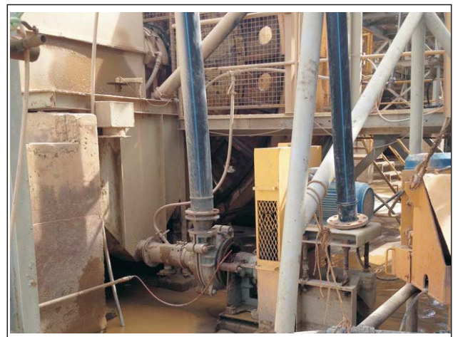
Mineral concentrate in a iron ore mine 4x3D-WX Q=144m 3 /h, H=38m, n=1960rpm, \gamma =1.13
