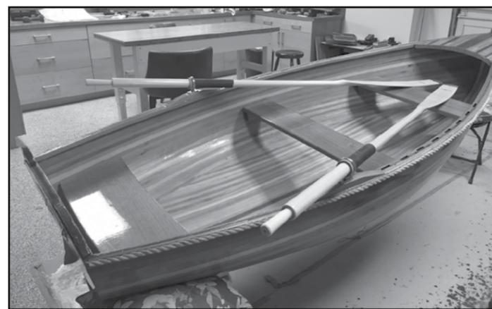
Two more coats of resin with ample sanding in-between to smooth drips and we were ready to add the gunwales, the boat's top railing. Gunwales are composed of two long pieces of wood called outwale and an inwale that are cut to fit, faired back from the bow and stern where they have to be thinner. We had a neighbor router the outwale to create the scooped-out
