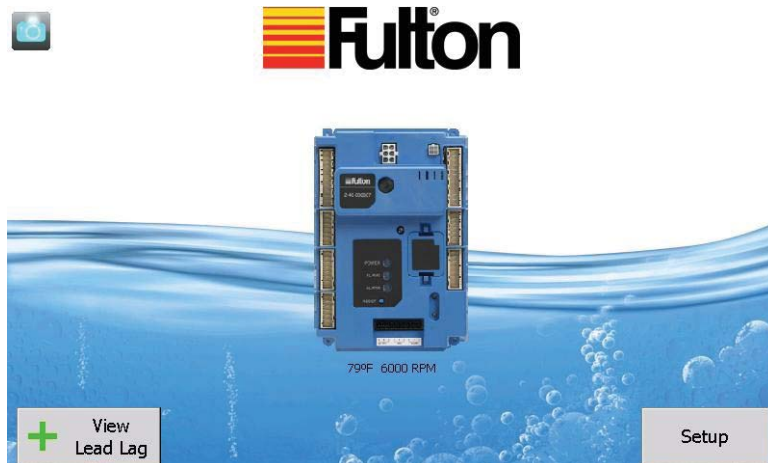
FIGURE 11 - THE SOLA CONTROLLER HOME SCREEN
