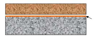
Aggrepave Polymer surface soaked 40 mm depth 6mm to dust aggregate layer Polymer surface sealed Driveway/ pathway
