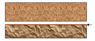
Aggrepave Polymer surface soaked 80mm depth 6mm to dust aggregate layer
