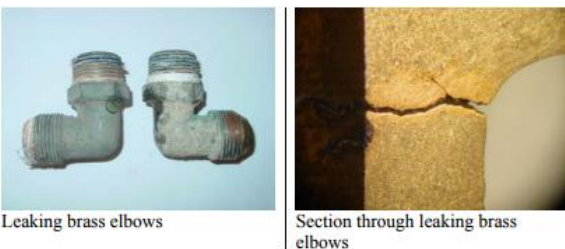
Figure 13: Cracks in Brass Elbows (WSAA [6])
