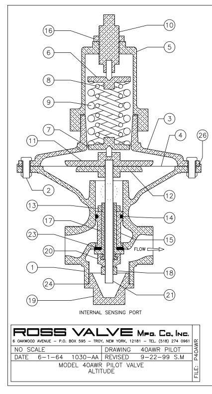
The purpose of a pilot valve is to control the opening and closing of the main valve by trapping or releasing water from the main valve's "operating chamber" ("K" - the chamber above the main valve piston). The **Model 40AWR Altitude Pilot Valve** uses this logic in order to maintain a constant pressure (water elevation) downstream of the main valve.
