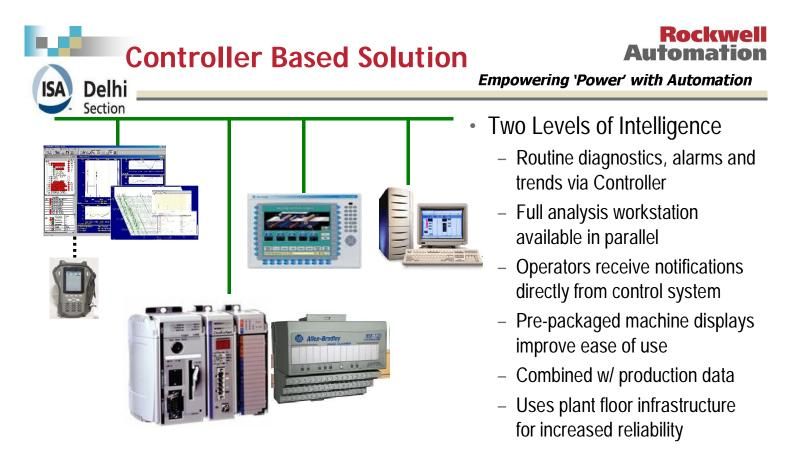
The Integrated solution collects data multiple times a day, analyzes using programmed rule sets and converts it to actionable diagnostic messages. This eventually takes away the burden of manually collecting and analyzing data. Both operations and maintenance personnel can be informed about specific pending machinery problems before they cause unplanned downtime.
