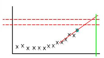
Example: Vibration level increasing with time.
