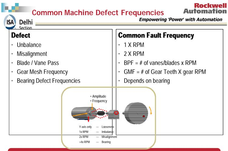
System can track 4 independent bands and Fault Frequencies
