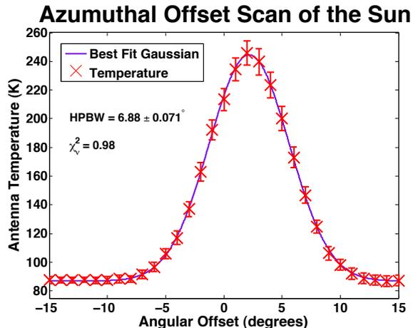
FIG. 3. 6 reduced azimuthal scans of the sun between offsets of  $-15^\circ$  and  $15^\circ$  at 1420.4 MHz. The errors were the standard deviation of temperature at each offset divided by  $\sqrt{n}$ . We fit a Gaussian to this data and determined the maximum relative antenna temperature to be  $156.62 \pm 1.99$  Kelvin. We took the difference between the center of the peak and  $2\sigma$  and find the HPBW to be  $6.88 \pm 0.071^\circ$ .
