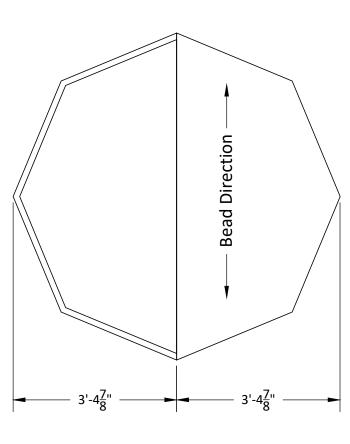
Bottom View-Must be removable, will notch for posts and install at load in.
