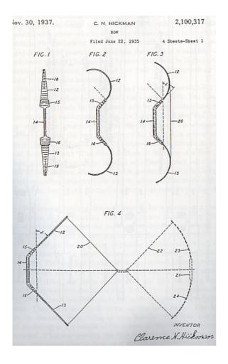
This is a copy of illustrations from Clarence Hickman's patent application of 1935. This shows the un-strung and strung bow in the top pictures and then in the lower illustration, the shape it takes up when brought to full draw. As can be seen, this has a narrow hand grip and low brace height, because it was intended initially to be used for Flight Shooting. It therefore adopted characteristics from the Turkish flight bows.
