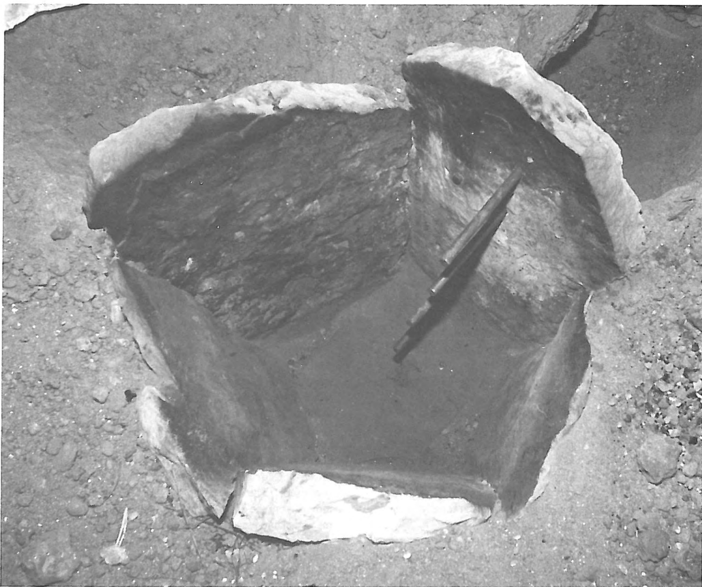
Figure 4: Experimental slab-lined fire pit with probe wells installed for taking temperatures.
