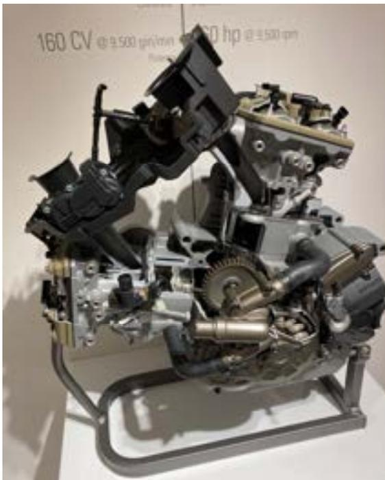
The 2014 Ducati Testastretta DVT 1200 cc engine. Its variable timing adjusted power needs based on RPM.
