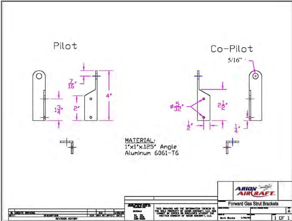
the instrument panel. Use the 1/8" thick aluminum angle supplied in the kit.
