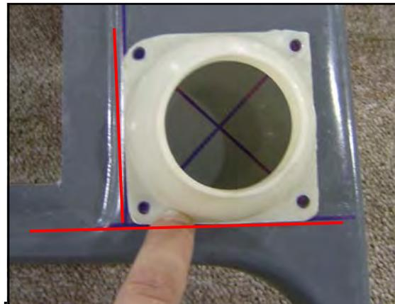
18. Match drill the holes in the flange thru the panel box with a 5/32" drill bit.
