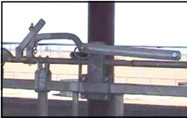
**Pivot Bar Between Latching Sleeves**
