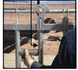
11. Go back to the handle and set it to the Self-Locking position. Measure the distance between the stationary Vertical Fence Bar and the Pivot Bar. Refer to the chart below to ensure that the measurement is correct. This distance should be the same at the top and bottom.
