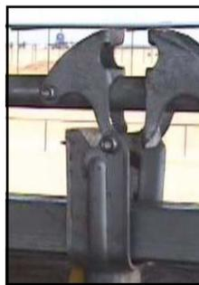
**Latching Sleeves Perfectly Aligned**
