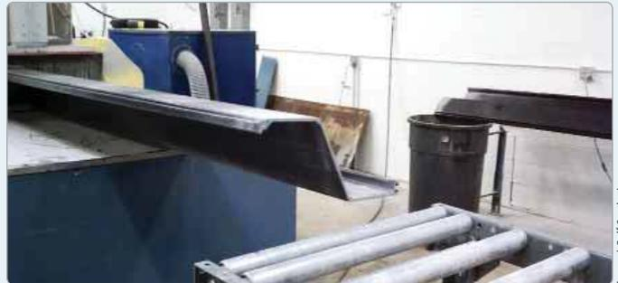
8 The Gulf profiles are pultruded at a rate under 2-ft/min (0.61m/min). An automatic, flying cut-off saw cuts the profiles to the specified length for each job. ■
