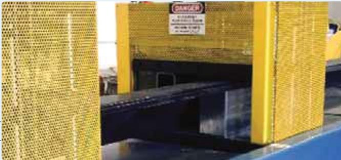
7 Clamp pressure is adjustable and separate from pull load pressure, which reduces the incidence of cracking profiles. ■
