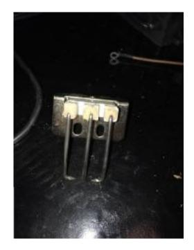
Remove old wires from Needle
