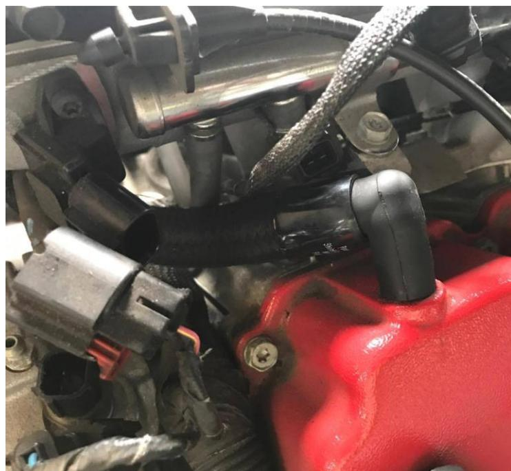
**DSE Gen III catch can installed (left) showing driver side valve cover exit (right)**
