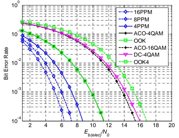
Figure 7. BER as a function of  $E_{b(elect)}/N_0$  for PPM, OOK, ACO-OFDM and DC biased OFDM.
