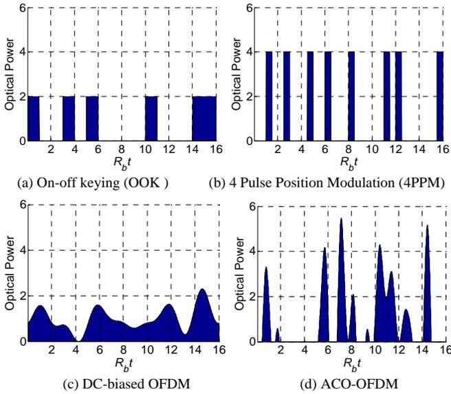
Figure 5. Time domain waveforms
