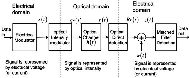
Figure 1. Intensity modulated/ direct detection optical communication system.
