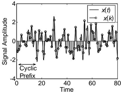
Figure 3. Bi-polar OFDM signal (64 subcarriers, cyclic prefix length of 16)
