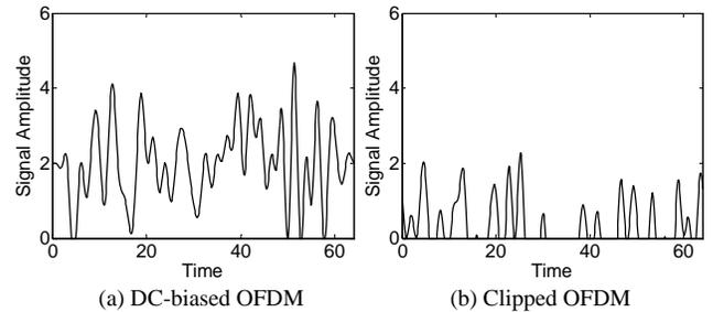
Figure 4. Transmitted optical signal for DC-biased OFDM and ACO-OFDM
