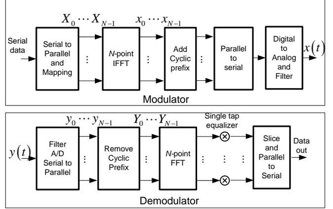
Figure 2. Block diagram of an OFDM communications system.
