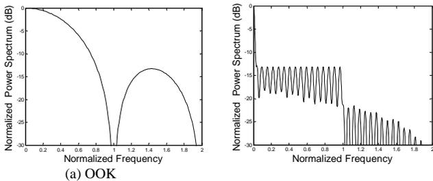
Figure 6. Power spectrum of OOK signal on linear and dB scales.
