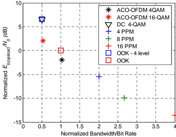
Figure 8.  $E_{b(optical)}/N_0$  for a BER of  $10^{-3}$  versus normalized bandwidth for PPM, OOK, ACO-OFDM and DC biased OFDM.
