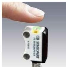
**F10 Photo-Eye** comes with fixed focus red LED or teach-in laser capabilities; NPN/PNP; N.O./N.C.; IP-67; Switching Frequency ≤ 1000 Hz; Response Time 500 μs; Operating Voltage 10 ... 30V DC; Material Housing/Screen: PUR/PMMA
